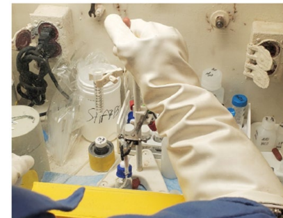
Loading resin contacted with Ra-224 to fabricate a generator
