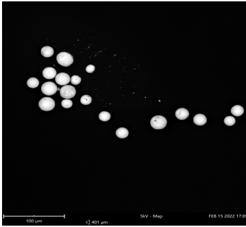
Precision dispensing: 19 Tungsten powder particles totaling 21 \mu\text{g}
