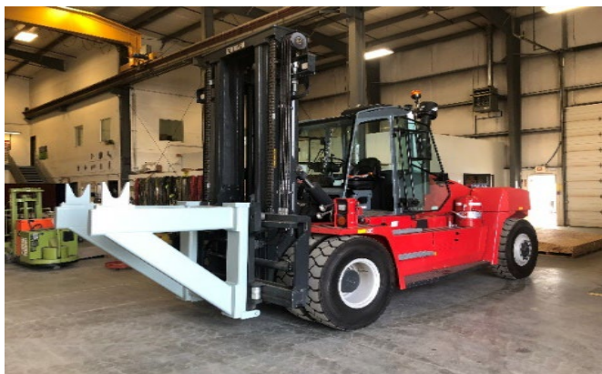
Modified Forklift to Safely Lift and Transport 27,000-pound Self-Shielded Ion Exchange Columns
