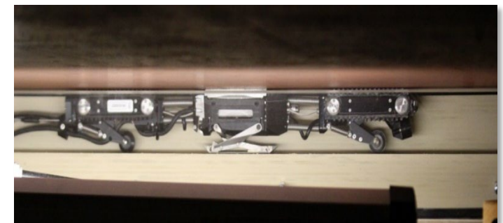
Remote Air-slot Volumetric Inspection System
