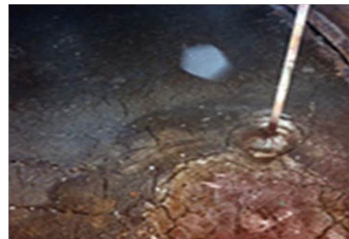
Water-insoluble metal oxides, significant amount of interstitial liquid - texture similar to peanut butter
